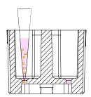
! Critical Lay the plate on a flat surface while seeding cells into the organiX plates. Inclination of the plate affects the flow in the media channel, thus disturbing cell distribution.
