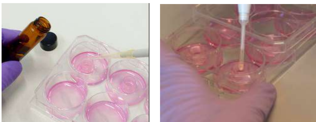
Figure 2: Application of normal liquids with a standard pipette (left) and viscous liquids with a positive displacement pipette (right).
