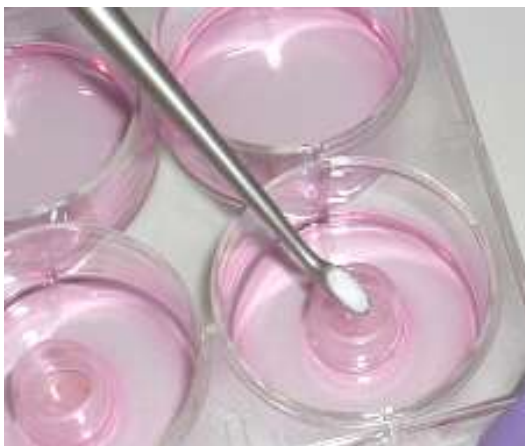
Figure 5: Application of solids.
