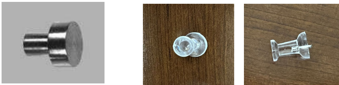
Figure 7: The stainless steel aid or push-pin (with metal spike removed). Both can be used for application of waxy materials following sterilization with 70% ethanol.
